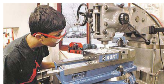
Ithaca High School sophomore Ravi Lal operates a mill during a work session for Code Red robotics. D.W. NUTT / STAFF PHOTO
